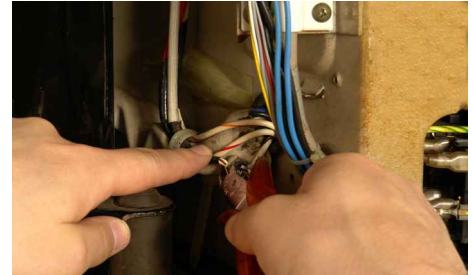
6 Cut connection between thermostat and compressor
