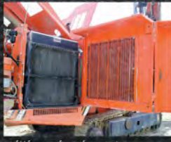
Drilling Rig Air Intake
